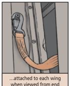
...attached to each wing when viewed from end with personnel door, and all damaged straps replaced before unlocking cam locks on side wings
